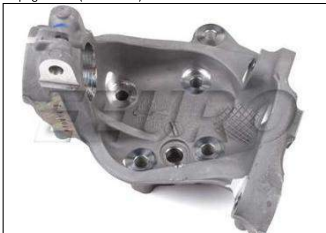
PHOTO 46 Upright front (inside view)
